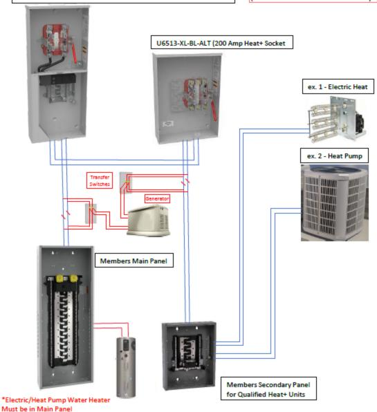
All wiring must meet current NES Code and Electrical Inspections
