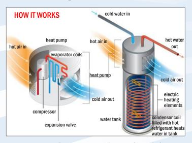
Heat pump water heaters come with control panels that allow you to select from different operating modes:
