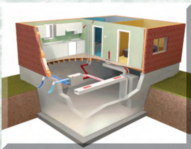
A continuous, balanced ventilation system brings in fresh air from the outside while exhausting stale air from the inside.
