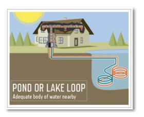
Pond or lake loops are economical to install. Coils of Polyethylene tubing are simply placed on the bottom of the pond or lake.
