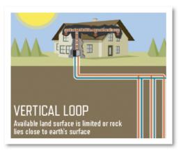
Vertical loops use drilling equipment to bore smalldiameter holes from 50 to 200 feet deep. Polyethylene tubing is then fed down these holes creating a loop pattern. The individual loops are all joined together and tied to the indoor heat pump unit.
