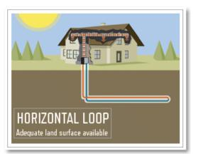
Horizontal loops are trench into the ground below the frost line with Polyethylene tubing (300-600 feet of trench per ton). The majority of horizontal installations in Iowa use a slinky coil loop. This design allows three times the amount of pipe to be installed (laid upright or flat) in a trench. Horizontal loop requires more land, but has a lower installation cost.
